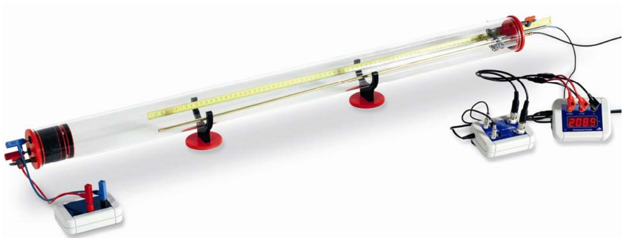
Fig. 1 Determination of speed of sound by measuring the time it takes for a sound pulse to cover a given distance
