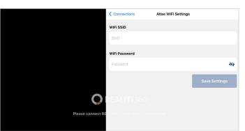
**6.** After entering the desired Wi-Fi SSID and password, tap 'Save Settings' to apply the changes successfully to the Wi-Fi configuration.
