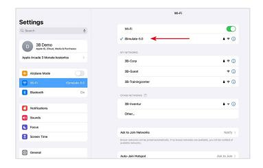
3. Turn On Atlas Baby: Locate and press the power button on the back of the manikin. This will automatically connect it to the iSimulate-5.0 network. Once the connection is successful, the power button will change from yellow to green.
