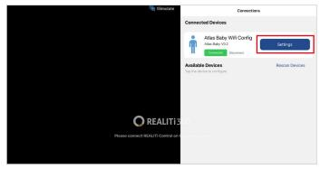
5. Rename Wi-Fi SSID: The Atlas Wi-Fi settings will show up, allowing you to customize the Wi-Fi network name to match your router. Ensure that both the Wi-Fi SSID (name) and password align with your Wi-Fi router.
