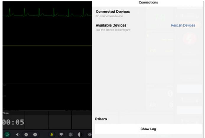
10. From the available devices select 'Atlas Baby' by tapping 'Connect Device'. The connected Atlas Baby will be calibrated automatically.
