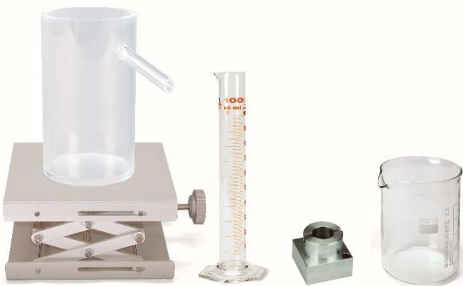
Fig. 1: Set-up for determining the volume of an irregularly shaped body
