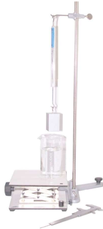
Fig. 1: Determining the updraught on a block
