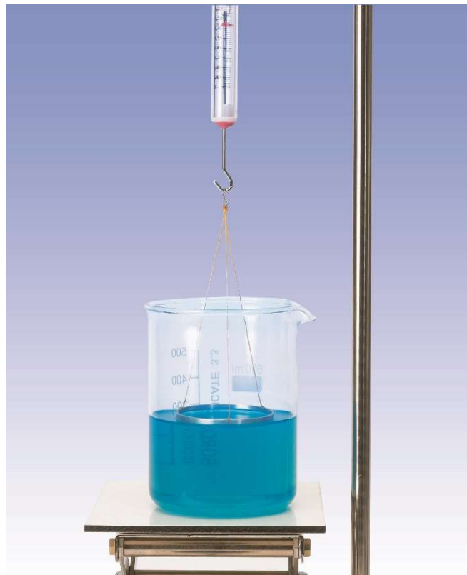
Fig. 3: Experiment set-up for surface tension measurements
