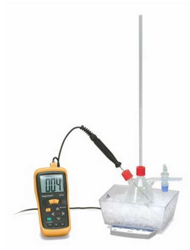
Fig. 2: Experiment set-up for determining the temperature of the maximum density of water
