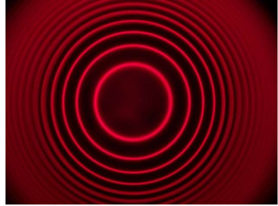
Fig. 7: Live image with Fabry-Pérot etalon
