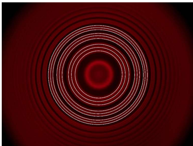
Fig. 5: Triplet splitting of the red cadmium line ( I = 5.0 A \triangleq B = 458 mT ). Interference rings marked with circles to determine the enclosed areas
