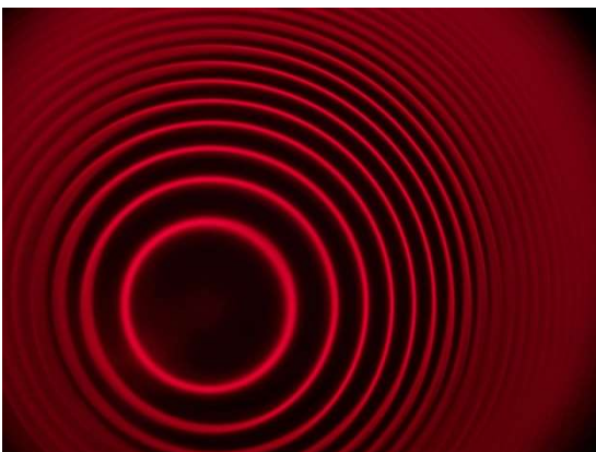
Fig. 7c: Etalon tilted. Correction: Adjust using the three adjusting screws on the housing.
