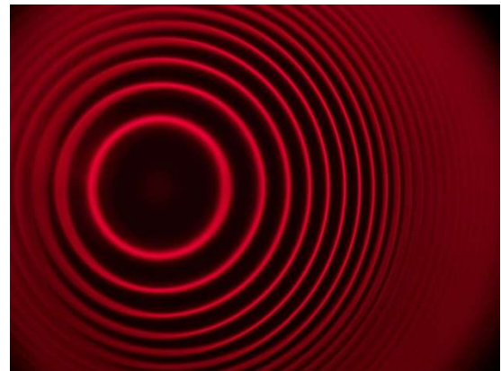
Fig. 7b: Etalon twisted in the optical rider. Correction: Rotate the etalon in the optical rider so that it is aligned perpendicular to the optical axis
