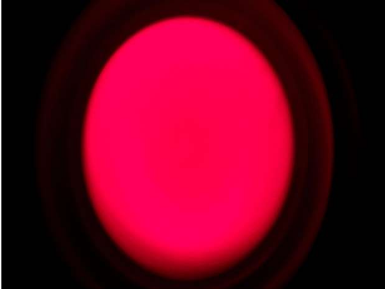
Fig. 6a: Condenser lens twisted in the optical rider. Correction: Rotate the condenser lens in the optical rider so that it is aligned perpendicular to the optical axis
