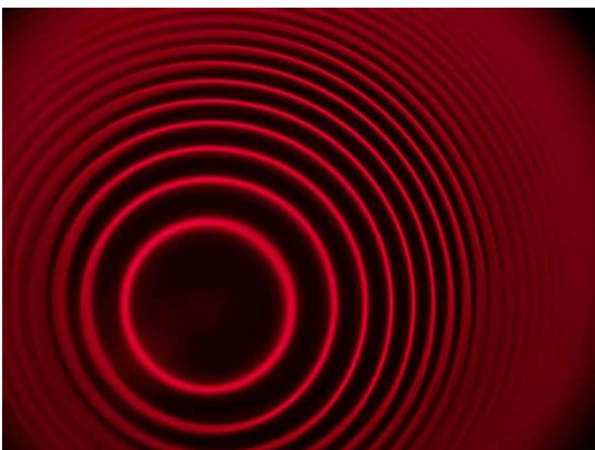
Fig. 7c: Etalon tilted. Correction: Adjust using the three adjusting screws on the housing.
