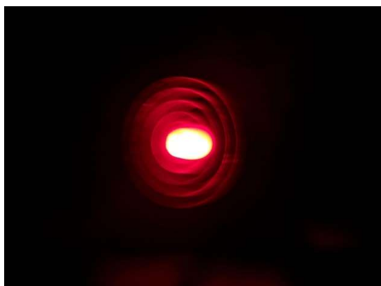
Fig. 5d: Imaging lens twisted in the optical rider. Correction: Rotate the imaging lens in the optical rider so that it is aligned perpendicular to the optical axis
