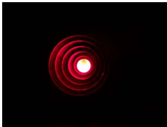
Fig. 5a: Electromagnet twisted. The stepped hole does not appear concentric. Correction: Turn the electromagnet so that it is centered
