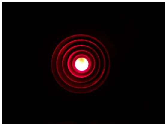
Fig. 5: Live image with camera and imaging lens. Stepped hole of the pole piece and light spot of the Cd lamp appear concentric and centered
